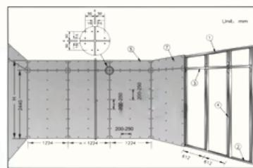
1. Top Track 2. Floor Track 3. Horizontal Keel 4. Metal Studs
